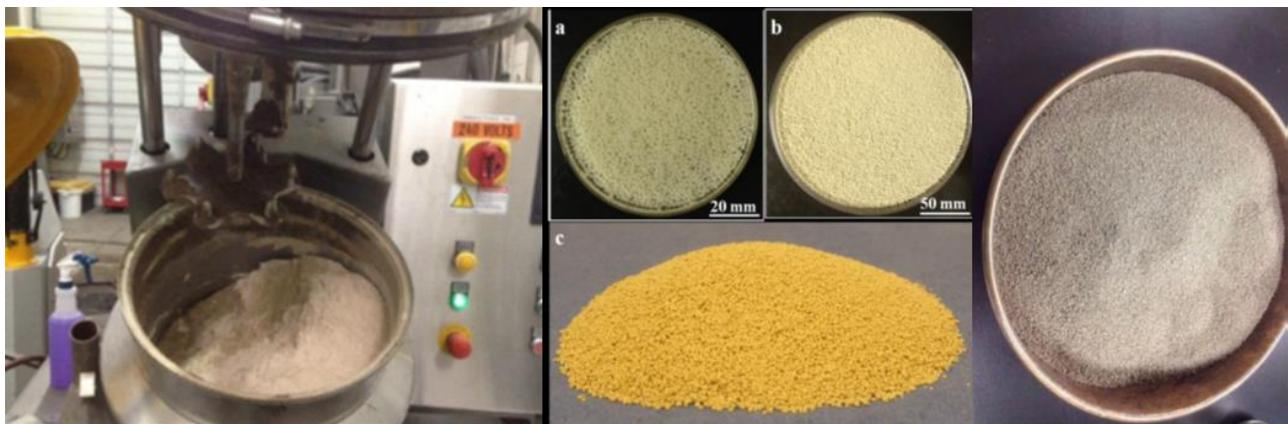
**Fig. 2. Geopolymer based-Proppants**
