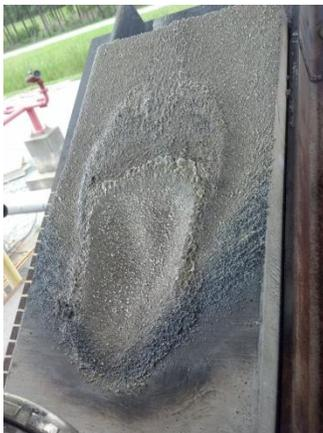
High Temperature Geopolymer panel tested at 4000°F at NASA Stennis.
