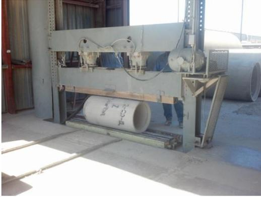
Geopolymer pipe about to be tested for D-load.
