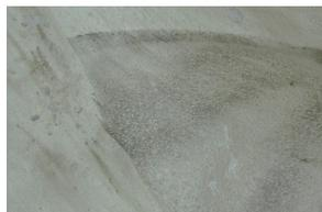
The geopolymer material was observed to erode/ablate at nearly identical rates as the surrounding commercial grade refractory material. There was no large-scale loss of geopolymer material and no indication of debonding of the geopolymer from the surrounding refractory of the concrete substrate. The geopolymer material has since undergone exposure to numerous subsequent engine tests with continued excellent performance.
