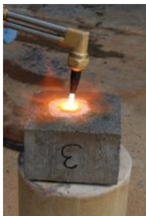
Figure 1. Geopolymer cube exposed to a flame of 1300°C.
