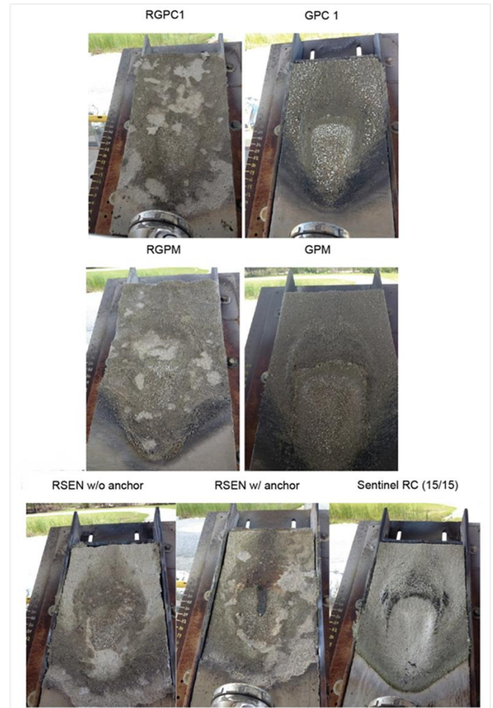
Figure 12. Repaired GPC1 panel (after 15/15 test) and original GPC1 panel (after 30/30 test). Repaired GPM with GPM panel (after 15/15) and original GPM panel (after 15/15) (middle). Repaired Sentinel panel without anchor after 15/15 test (bottom left), repaired Sentinel panel with anchor after 15/15 test (bottom middle) and original Sentinel panel after 15/15 test (bottom right).
