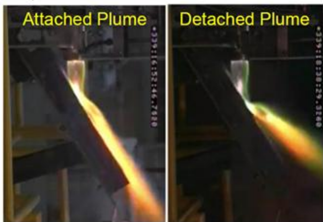
Figure 6. Example of Plume Detachment after Excessive Panel Erosion
