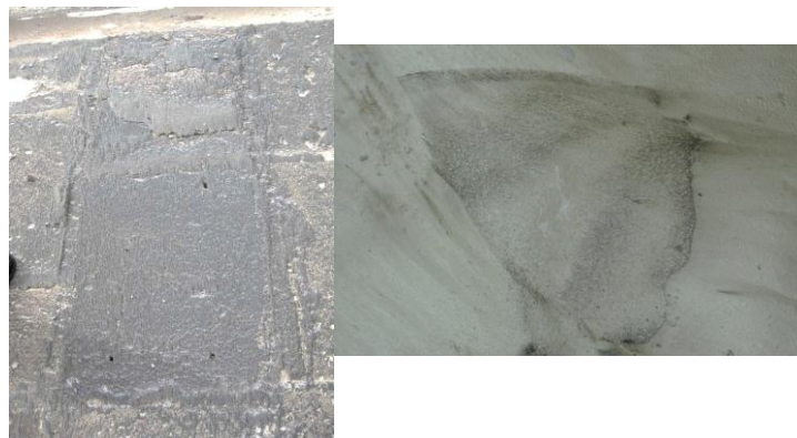
Figure 3. Geopolymer sections after rocket engine test.
